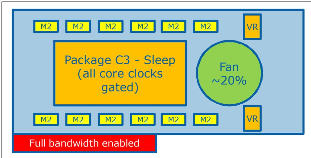
From M1 state, memory can be put in self-refresh mode to enter the M2 state, further reducing memory power.
