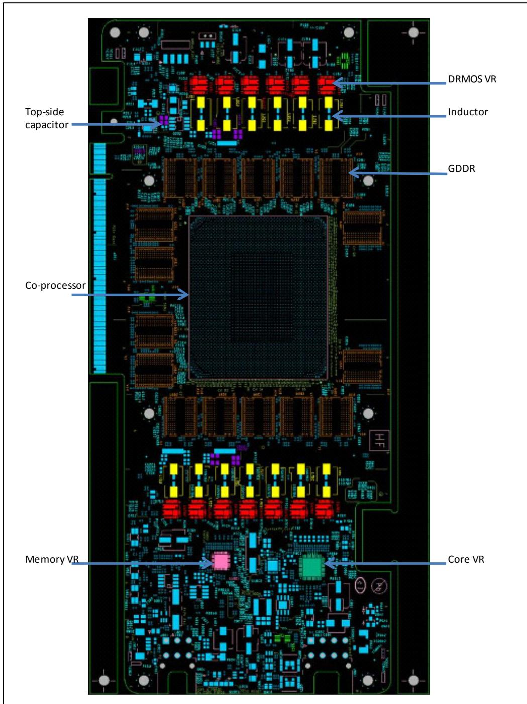
Figure 3-19 SE10X/7120X Board Bottom Side
