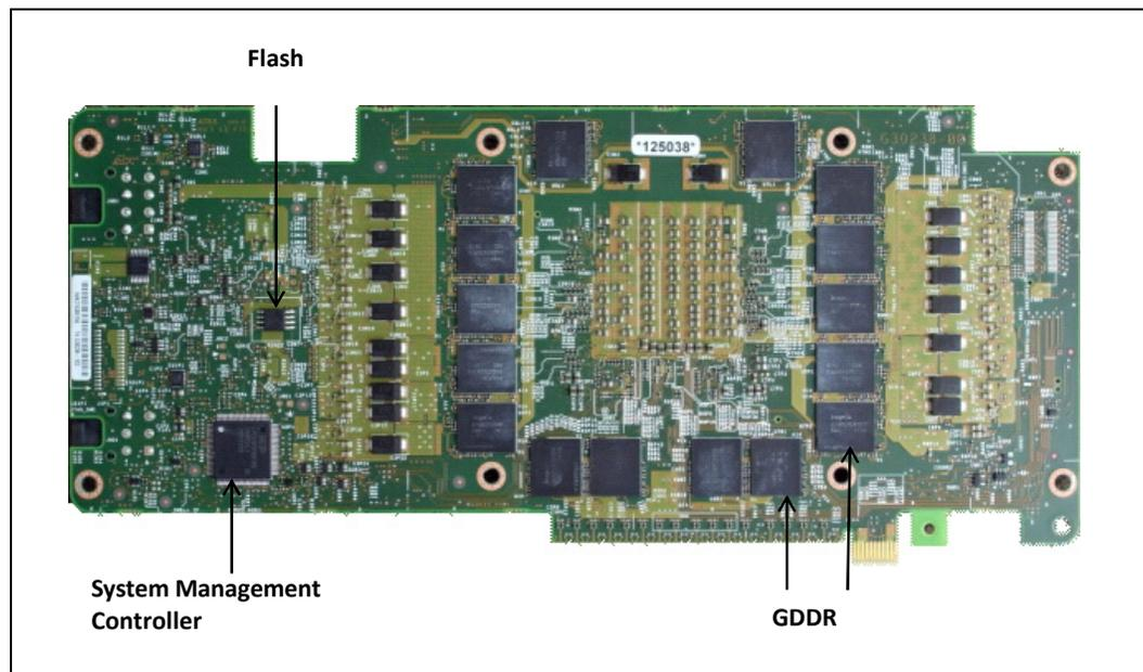
**Note:** Figure 2-2 and 2-3 are representative of the final Intel® Xeon Phi™ Coprocessor board without the package thermal and mechanical solution.
