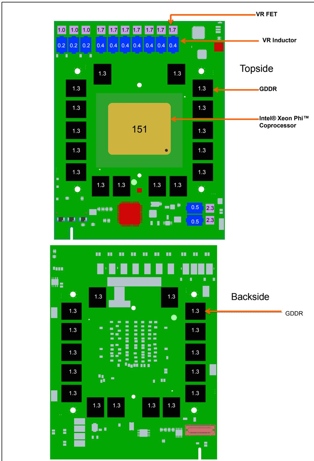
**Figure 3-12 5120D Power Profile: Memory Centric (all values in Watts)**
