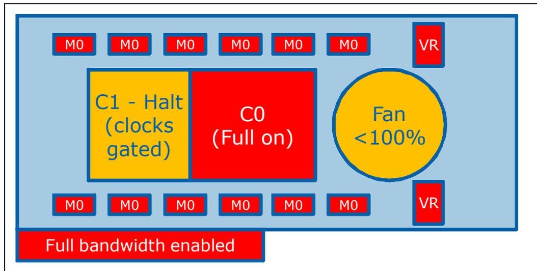
Coprocessor C1 state gates clocks on a core-by-core basis, reducing core power. On the active SKU, the fan slows to an appropriate speed, reducing fan power. If all cores enter C1, the coprocessor automatically enters Auto-pC3 state.
