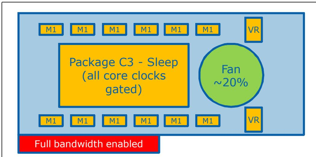
When all cores have entered C1 Halt state, the coprocessor package can reduce the core voltage and enter Deep-pC3. The fan (on active SKUs) can slow to minimum speed. VRs enter low power mode.
