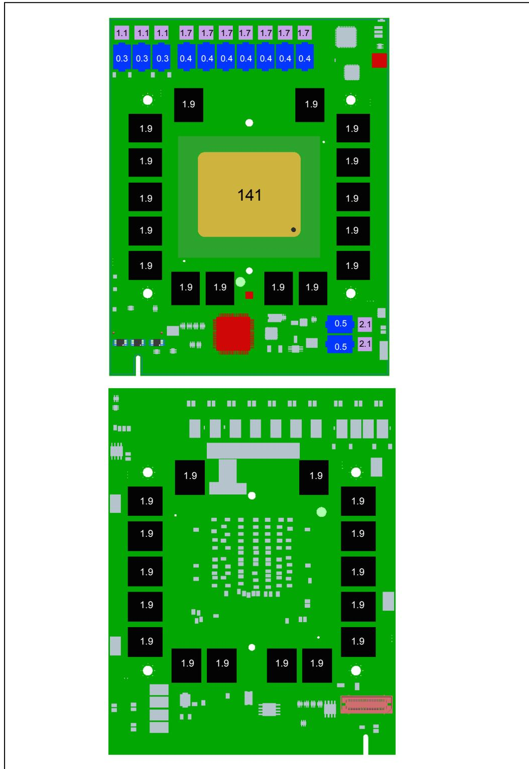
**Figure 3-14 7120D Power Profile: Memory Centric (all values in Watts)**
