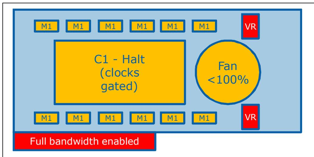
If clock-enable input to memory is pulled high, then memory enters M1 state which reduces memory power.
