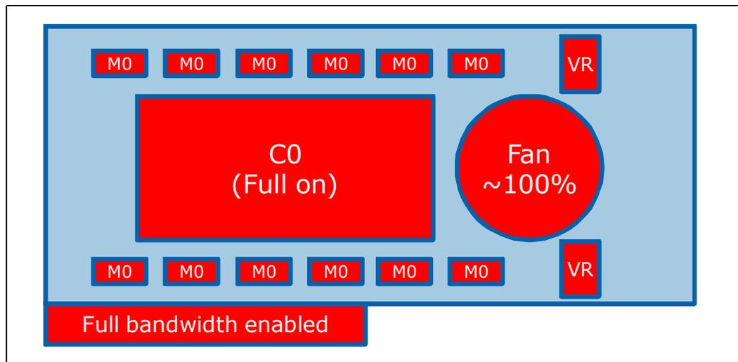
In this power state, the card is expected to operate at its maximum TDP rating.
