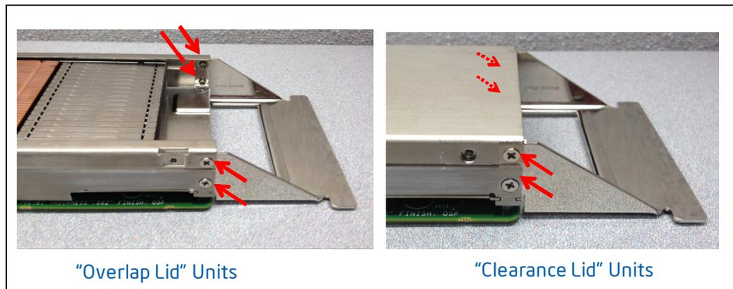
At this point, "clearance lid" units are ready to be mounted in the chassis.
