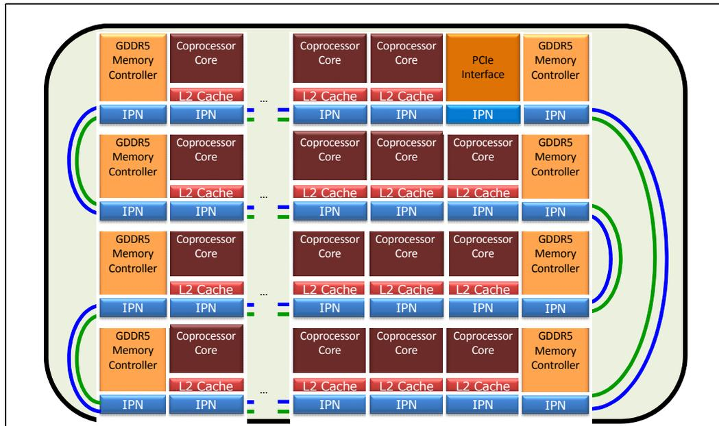
Figure 2-4 is a conceptual drawing of the general structure of the Intel® Xeon Phi™ coprocessor architecture, and does not imply actual distances, latencies, etc. The cores, PCIe Interface logic, and GDDR5 memory controllers are connected via an Interprocessor Network (IPN) ring, which can be thought of as independent bidirectional ring.
