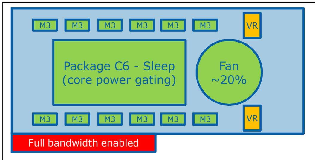
The memory clock can be fully stopped, reducing memory power to its minimum state.
