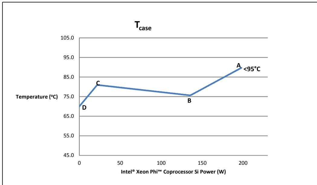
For the region A-B, the cooling solution must maintain the case temperature below 95°C which will in turn maintain the coprocessor silicon junction temperature below 104°C. Assuming an air-cooled heat sink, at a maximum coprocessor power dissipation of 198W (Figure 3-9) and an inlet air temperature of 45°C, the following equation between coprocessor junction-to-case and case-to-air heat sink rating can be used to determine the minimum necessary performance of a cooling system:
