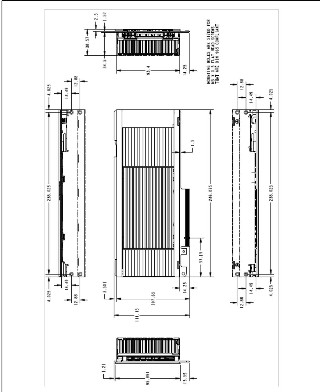
**Figure 3-2 Dimensions of the Intel® Xeon Phi™ Coprocessor Card (in mils)**
