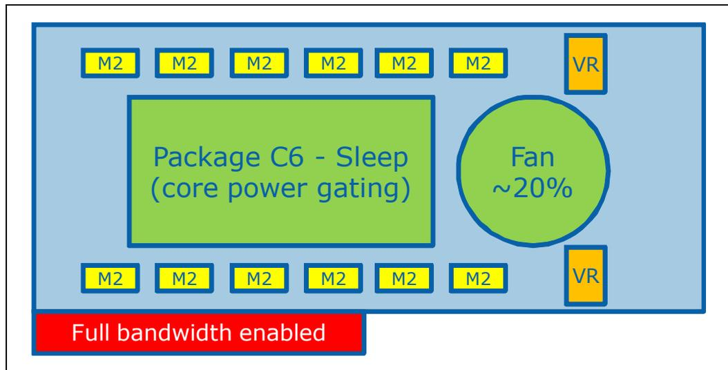
The coprocessor OS can request that the coprocessor enter package C6 state. Core voltage is shut down. Coprocessor power is  $<10W^1$  in this state.
